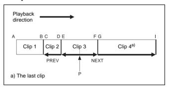
When you press the PREV button or the NEXT button at the current position (point P), the unit behaves as follows.
